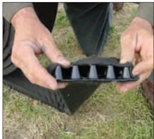
3-dimensional, high-flow drainage core
